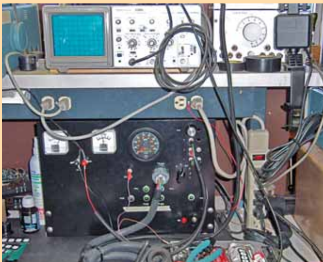
The HGM partners constructed this bench-test machine to give every unit a full battery of tests before being packaged and shipped.
