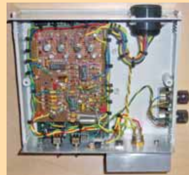
The original prototype CompuShift was wired and hand-soldered on a breadboard.
