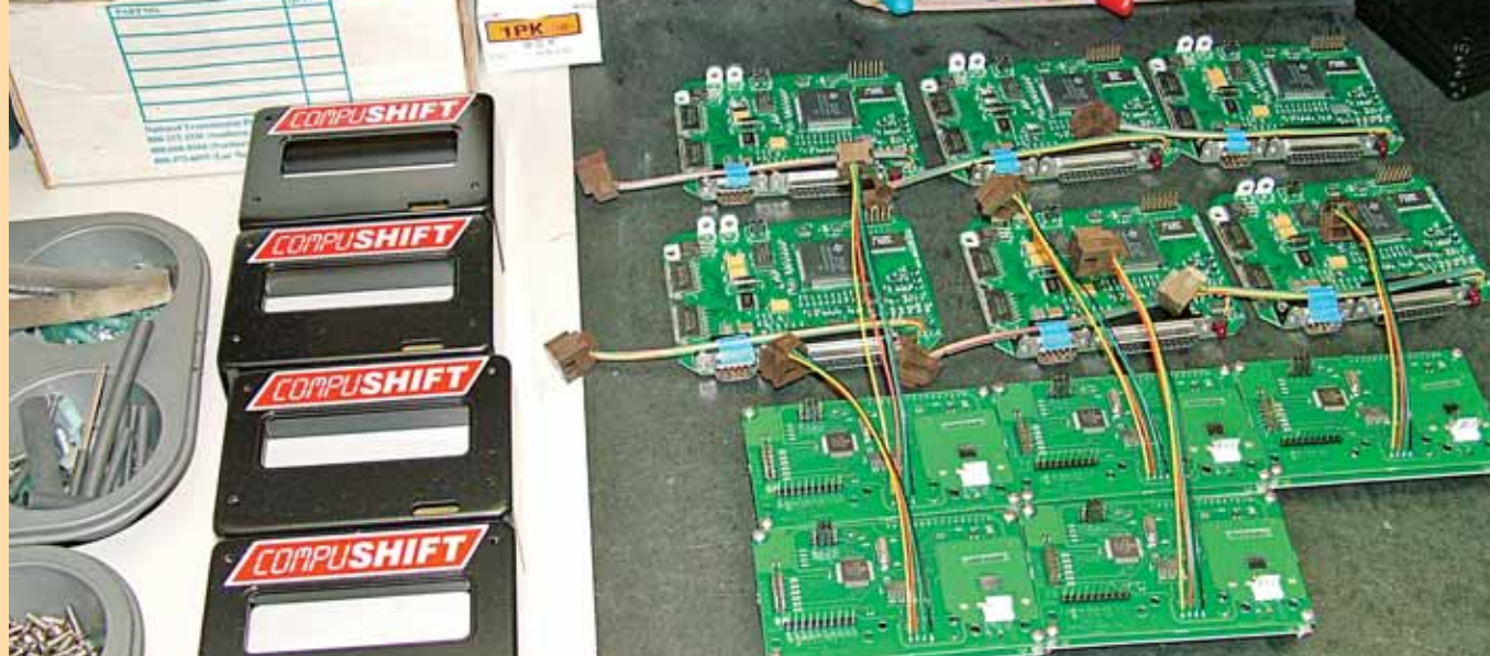
Component boards, the heart of CompuShift, are readied to be tested and assembled.
