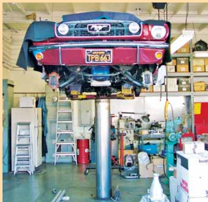
A 1966 Mustang is receiving a complete re-power. It gets a new 5-liter crate engine, CompuShift-controlled 4R70W, a new differential setup, exhaust system and rewiring.
