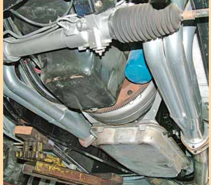
A bottom view of a 1960 Buick convertible with a 502 Chevrolet crate engine, 4L80-E and a 3.55-1 differential. Before the CompuShift modifications the car churning 3,000 rpm at highway speeds; after the changeover the range is 2,000-2,200 rpm.
