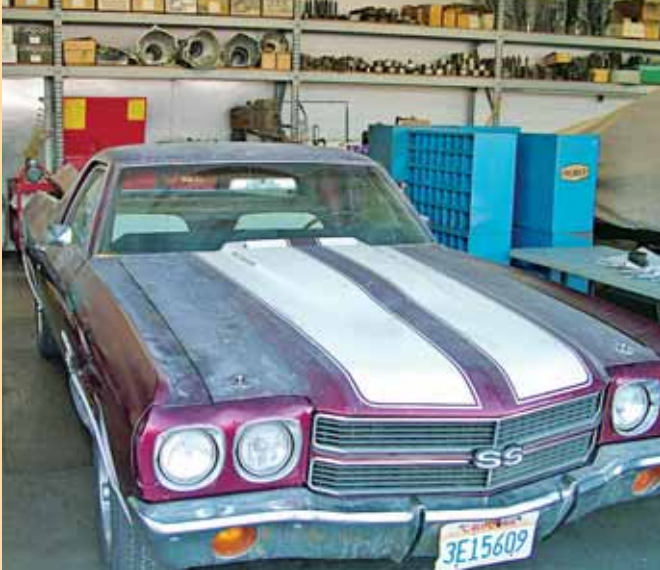
This El Camino has a built 454 engine replacing the original 400. That vehicle didn't like highway driving, so a 4L80-E transmission was installed. Adding the electronic transmission means that it can be driven on the freeway without being tied to the engine speeds that would have applied to the original 400 engine.
