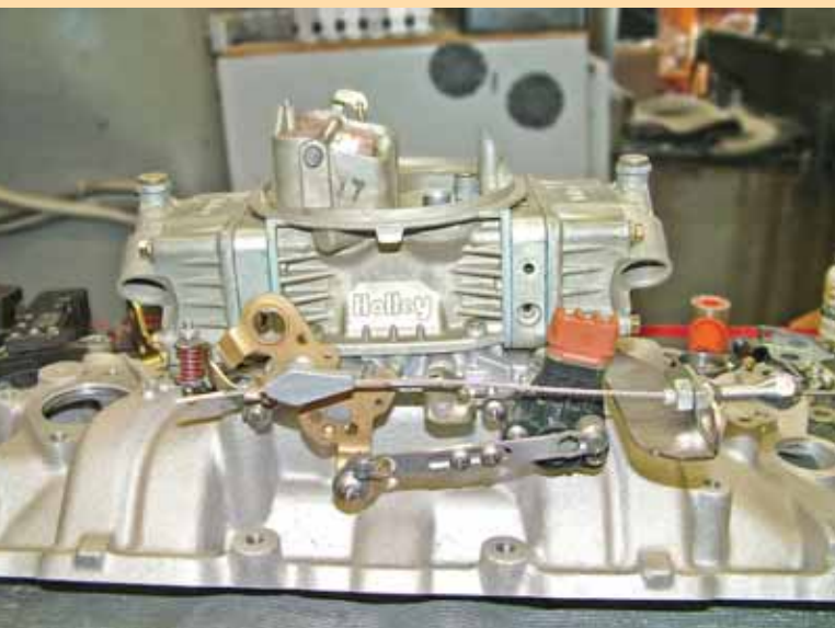
The AccuLink allows the CompuShift to acquire a TPS signal from carbureted engines.
